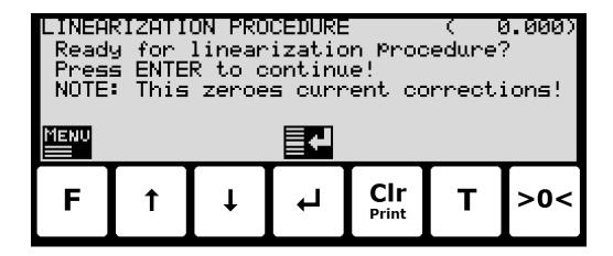
The different steps of the linearization procedure to be followed are described and listed in chronological order in the table below. Unless stated otherwise below the value shown in the upper right corner is the actual gross weight, corresponding to the gross weight shown in the **NORMAL** screen (with enhanced resolution selected).
