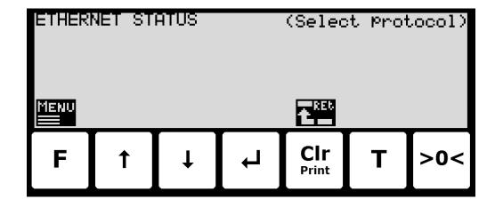
By use of the screen menu (the F key) the active Ethernet protocol, whose status is to be read, is selected. For an Ethernet protocol to be selected, it must be active. This means, that the protocol itself must be enabled in the **ETHERNET PROTOCOLS** screen (which again also may require, that the corresponding communication option must be enabled).
