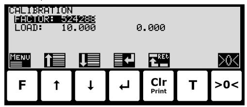
In this screen calibration parameters such as calibration factor, calibration load (to the left) and actual gross weight (to the right) are shown and can be changed. This makes it possible to calibrate the system. From the **CALIBRATE** menu it is possible to select the **CORNER CALIBRATION** screen for corner calibration of the system. A cursor (inverted text) indicates the currently selected parameter.
