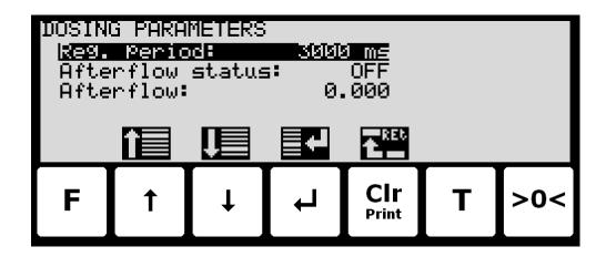
In this screen dosing parameters such as registration period and afterflow correction are shown and can be changed.
