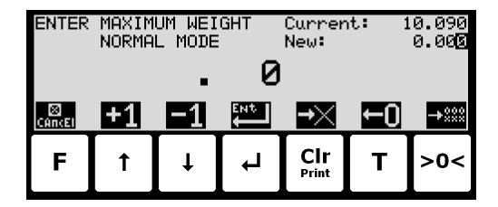
The actual parameter changed is indicated in the upper left part of the display. The current parameter value and the currently entered value is shown in the upper right part of the display. The currently entered value is also shown in the middle of the display in large font.
