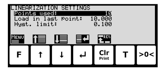
In this screen the **Points used**, **Load in last point** and **Hyst. limit** parameters (used for a possible linearization) are shown and changed. A cursor (inverted text) indicates the currently selected parameter.
