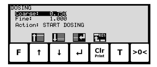
In this screen setpoints for dosing are shown and can be changed. It is also possible to start/stop a dosing.
