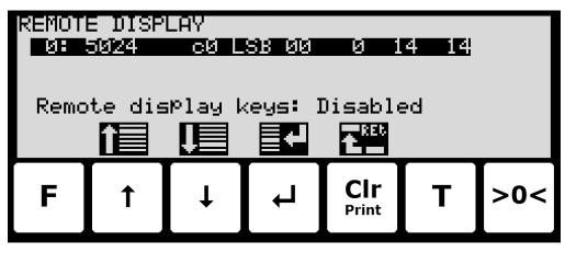
In this screen the enabled external devices are shown and can be changed. A cursor (inverted text) indicates the currently selected device. With this version of the software only one remote display can be installed.
