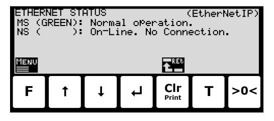
This requires that the EtherNetIP protocol is selected from the menu (the F key) in the **ETHERNET STATUS** screen. The currently selected protocol is shown in the upper right corner of the screen. If the **EtherNetIP** protocol is selected, then the EtherNetIP status indications for both Module Status (**MS**) and Network Status (**NS**) are shown, corresponding to the normal **MS** and **NS** lamps as follows:
