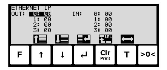
This screen will show the data sent to the EthernetIP master (*OUT*) and the data received from the EthernetIP master (*IN*).
