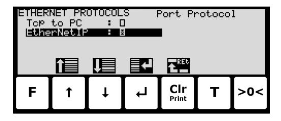
In the **ETHERNET PROTOCOLS** screen the '**EtherNetIP**' parameter is selected using the cursor, and *I* is pressed to enable or disable the Ethernet-IP protocol. A **X** in the corresponding box indicates the protocol is enabled. From the appearing menu it is also possible to switch to the **ETHERNET IP DATA** screen.
