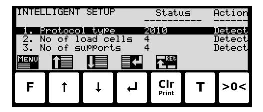
The screen shows a list of the different weighing technical parameters that the Intelligent Setup feature can try and detect. For every parameter in the list *Status* corresponding to the actual value of the parameter is shown, as well as *Action* corresponding to if the parameter is chosen to be detected (*Detect*) or kept unchanged (*Ignore*) during *SEMI* auto. detection. During *FULL* auto. Detection this column is ignored as it is assumed that *Detect* has been chosen for all parameters.
