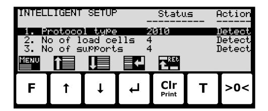
The screen shows a list of the different weighing technical parameters that the Intelligent Setup feature can try and detect. For every parameter in the list *Status* corresponding to the actual value of the parameter is shown, as well as *Action* corresponding to if the parameter is chosen to be detected (*Detect*) or kept unchanged (*Ignore*) during *SEMI* auto. detection. During *FULL* auto. Detection this column is ignored as it is assumed that *Detect* has been chosen for all parameters.
