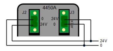
In an ATEX environment the 4x50 must be placed outside the hazardous zone and J3 must be supplied through the 4051A ATEX power supply:
