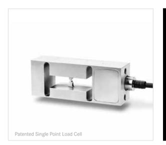
The Eilersen digital capacitive technology is based on an accurate and stable ceramic sensor, which is non-contacting and therefore unaffected by overloads, sideloads, torsion and welding voltages.
